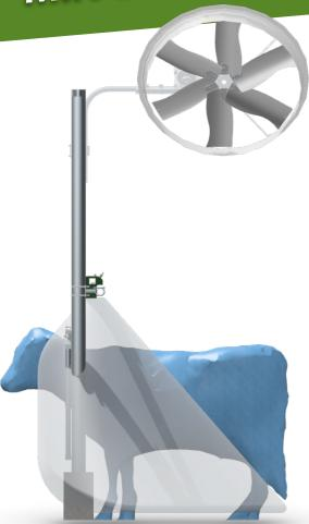
With standard soaker line height (1.8-2.0 meters) one unit will cover roughly 1.5 meters wide which is the standard coverage area per nozzle. Soaking cows during hot summer months will bring benefits. It reduces the impact of heat stress on the cows, improve their health and comfort, and increase milk production for farmers.
